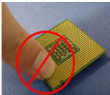
Open the Socket. Don't touch the processor contact.
