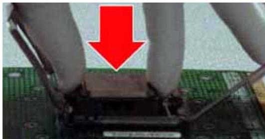
Carefully place the package into the socket body using a purely vertical motion.
