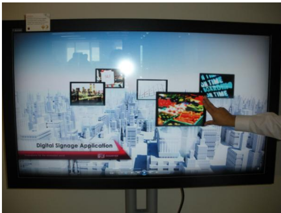
Figure 1: Intelligent e-Board system with Axiomtek OPS870 digital signage player
