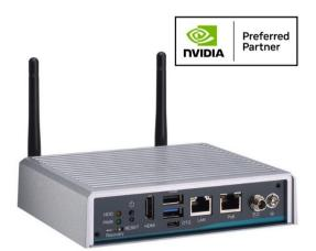
ready-to-deploy IP camera with both power and video transmission. It also has one M.2 Key M 2280 with PCIe x4 NVMe SSD slot for massive data processing. One full-size PCI Express Mini Card slot and one SIM slot are ready for 3G/4G, GPS, Wi-Fi, and Bluetooth connections.
